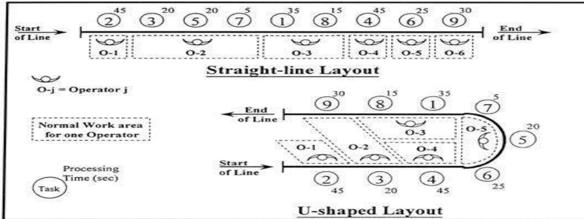
**Figure:** Product line or Assembly line layout (Line Processing Layouts)
